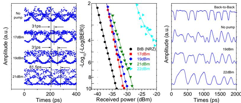
Fig. 7. Delay-time, eye diagram, BER and pulse pattern evolutions with pump power for the 10-Gb/s DPSK signal.
