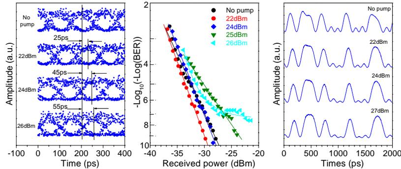
Fig. 6. Delay-time, eye diagram, BER and pulse pattern evolutions with pump power for the 10-Gb/s PSBT signal.
